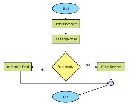
Figure 1.8: Activity Diagram with Decision and Connector Symbol
